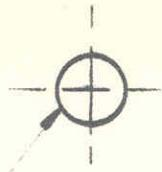
12 mm dia. hole for upper radiator mounting bolt
